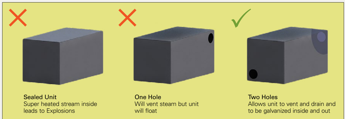
Figure 1: Purpose of Venting and Draining
