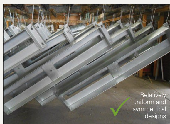
Figure 5: Avoid Distortion with Good Design
