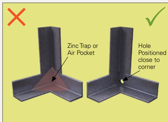
Figure 23: Inward Facing Angles – Venting Required
